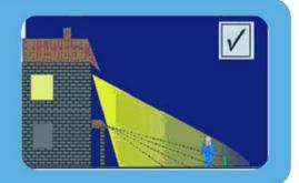
However, if possible use a separate detector that can be sited in a more ideal position where it is most likely to detect intruders into your property, rather than neighbours taking the dog for a walk or small animals roaming around the garden causing the light to switch on and off throughout the night.
