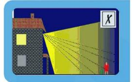
Unfortunately, many systems do not allow the detector to be separately aimed from the luminaire.
