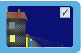
For many properties, a better solution for security lighting is to use a bulk-head or porch light fitted with a low power 600-900 lumens (9/11 w) compact fluorescent lamp.
